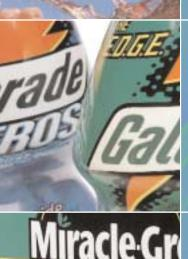
Shrink Sleeve Labels — This is the fastest growing segment of the label industry. Produced in colorful, cutting edge styles and materials, these alluring labels are manufactured as sleeves, slid over glass or plastic bottles and then heated to conform precisely to the contours of the container. Shrink sleeves can be found on many beverages such as Gatorade®. Our UniFlex division is one of the pioneers in shrink sleeve technology and positions us as one of the top suppliers nationally.
