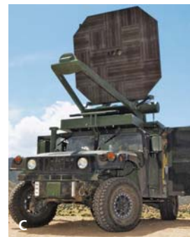
(A) A Raytheon Standard Missile-3 drew worldwide attention when it successfully brought down a non-functioning satellite in February 2008. (Photo courtesy of Department of Defense) (B) Excalibur brings next-generation precision to U.S. Army and Marine Corps artillery. (C) Active Denial uses millimeter-wave directed energy technology to create a zone of protection, repelling individuals without causing injury. (Photo courtesy of Department of Defense)
