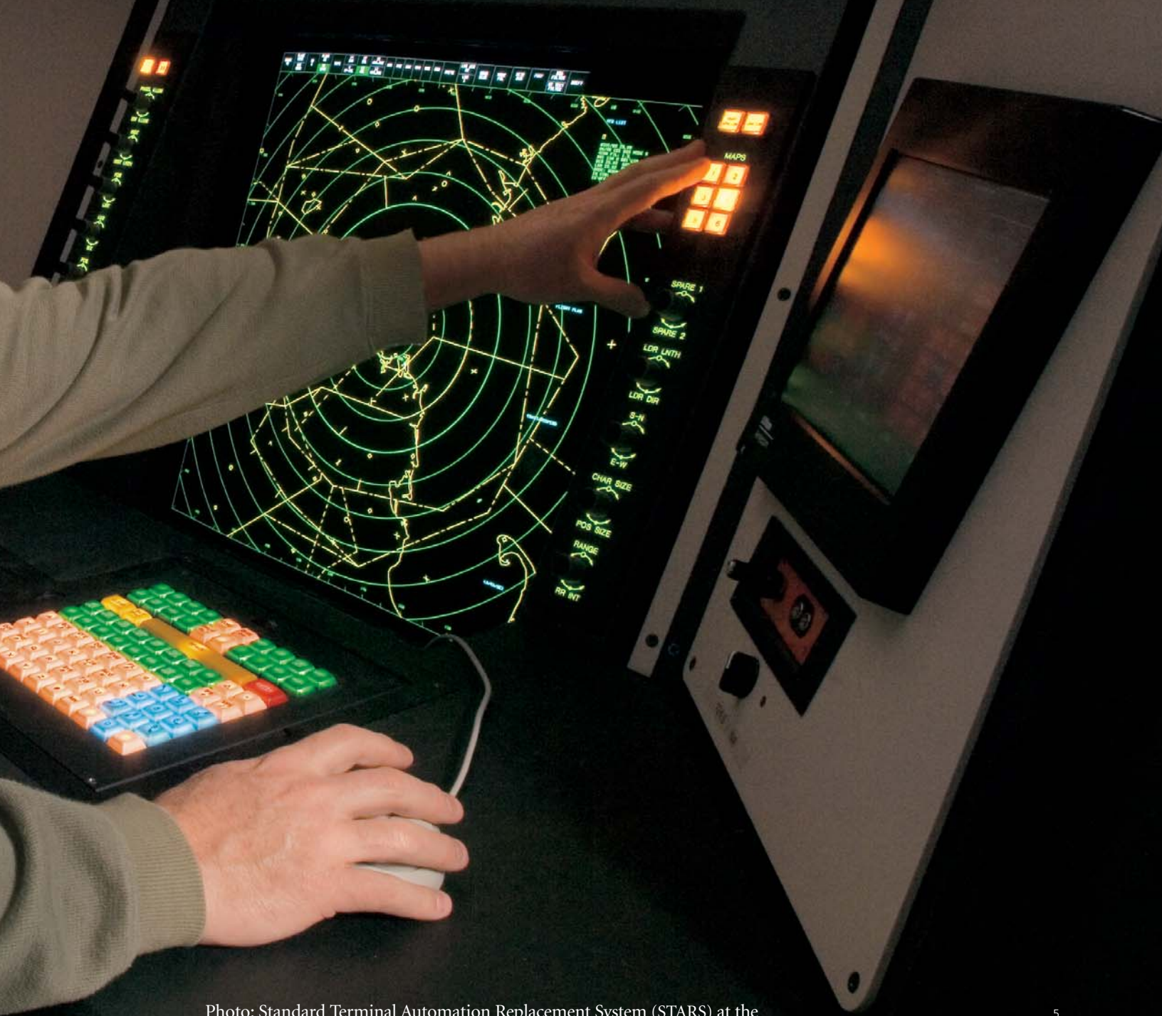
Photo: Standard Terminal Automation Replacement System (STARS) at the Boston Consolidated Terminal Radar Approach Control (TRACON)
