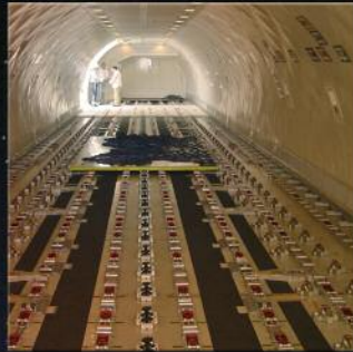
On-board cargo-handling system
