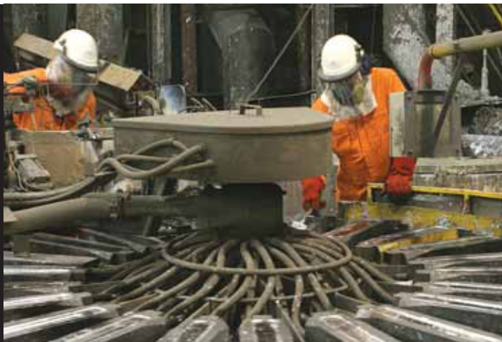
Recovering lead from batteries at ARA's facilities
