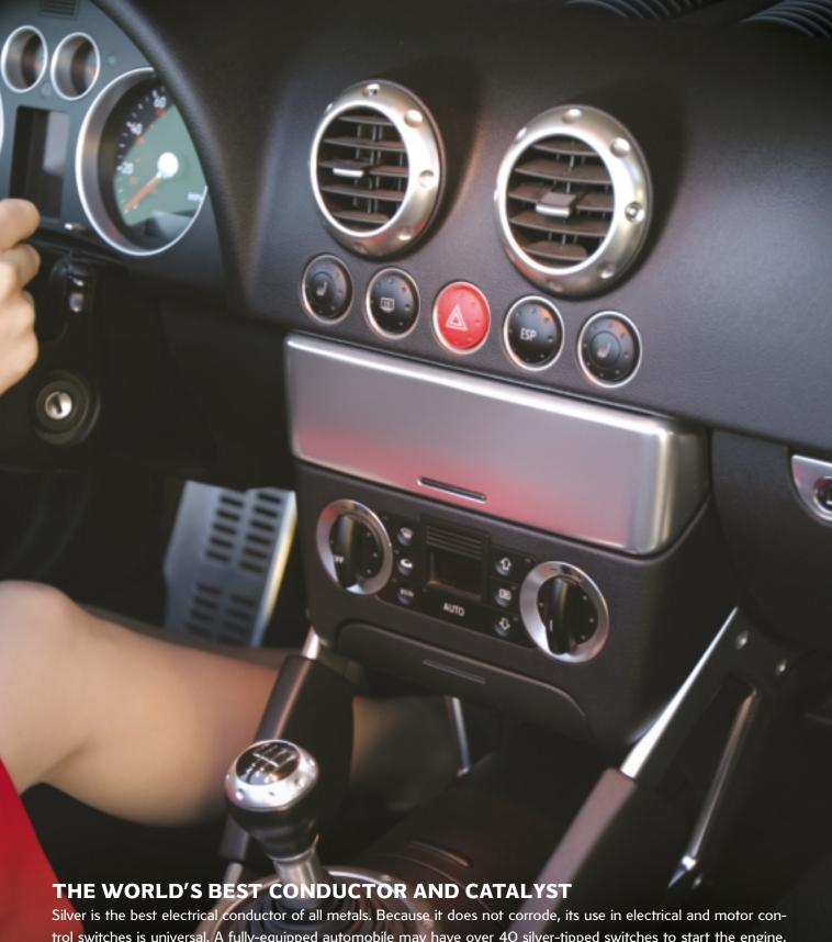
trol switches is universal. A fully-equipped automobile may have over 40 silver-tipped switches to start the engine, activate power steering, brakes, windows, mirrors, locks and other electrical accessories.
