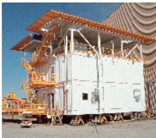
(Above) Shown here is the living quarters for Anadarko Tarantula, a fixed 4-leg production platform. The platform will be set in the Gulf of Mexico and has the capacity to produce 100 million cubic feet of natural gas per day and 30,000 barrels of oil per day. A variety of Ameron high-performance coatings were used throughout the platform.
