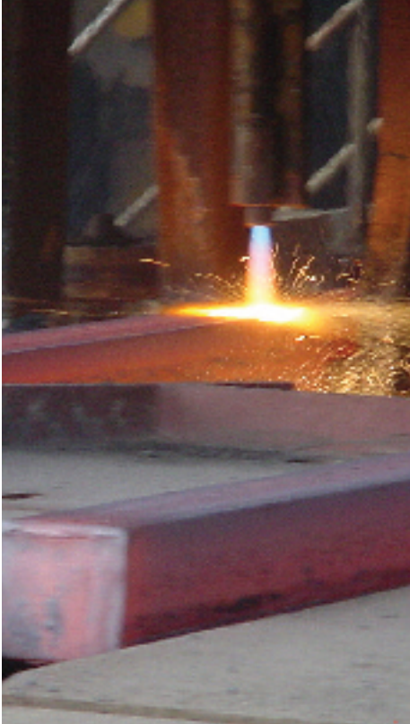
(Above) Automatic billet torch cutting at the continuous caster in TAMCO's steel mini-mill located in Rancho Cucamonga, California.
