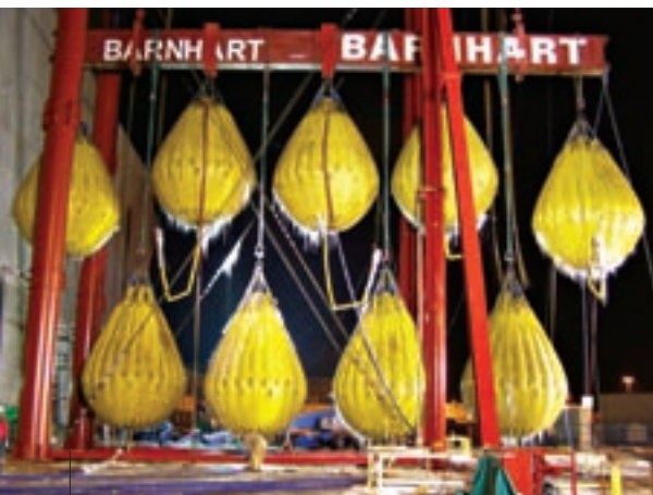
In sub-zero weather, ice forms on the expandable water-filled weights URS used to dead-load test the modular lift tower to ensure its ability to lift the giant MSRs.
