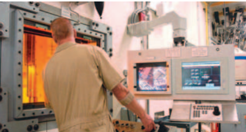
A URS facility operator uses a computerized workstation at a shield window to perform operations in the remote-handled waste facility.
