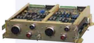
Electronic Power Distribution Center for Small Business Aircraft
