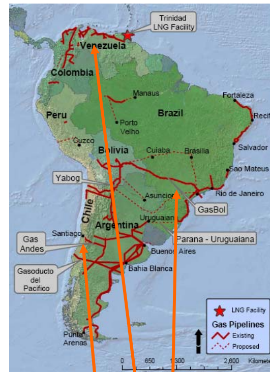
Gas network extensions In South America
