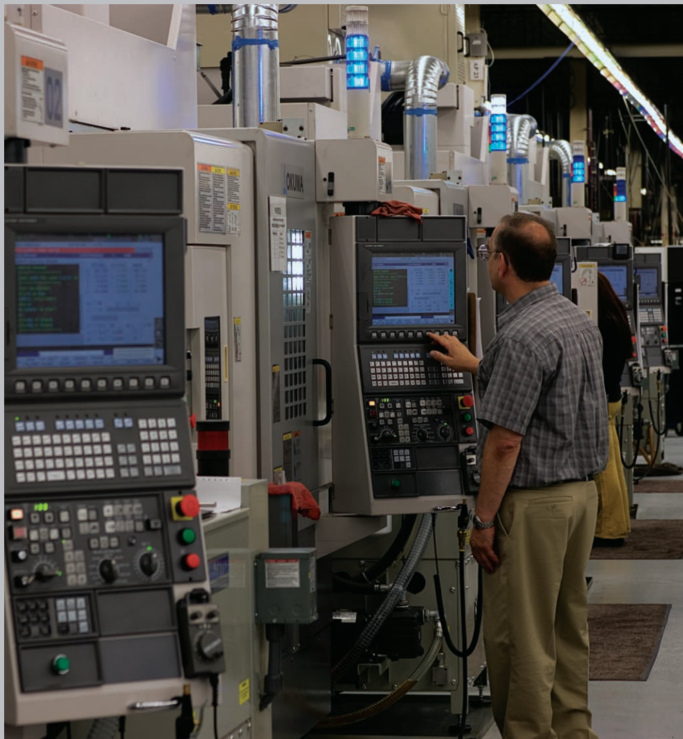
State of the art CNC machining centers, installed in fiscal 2007, produce high quality, lower cost revolver cylinders.
