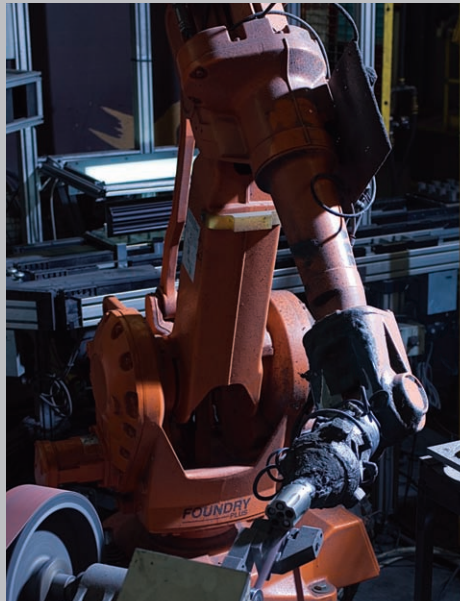
The robotic cylinder polishing process enhances both quality and output of revolvers.
