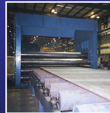
Multi-roll leveler flattens plates
