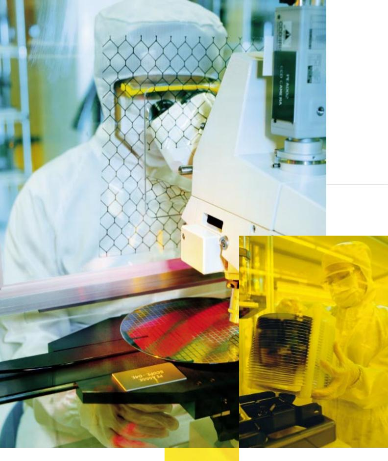
Wafers are visually inspected during the fabrication process as an extra quality check.
