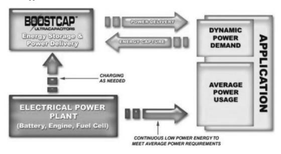
Although conventional batteries have been the most widely used component for both primary energy sourcing and peak power delivery, ultracapacitors, advanced batteries and flywheels now enable system designers to separate and optimize these functions. Based in part on our ultracapacitor products' rapidly declining cost, high performance and "life-of-the-application" durability, they are becoming a preferred solution for many energy storage and power delivery applications.
