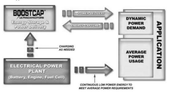
Although conventional batteries have been the most widely used component for both primary energy sourcing and peak power delivery, ultracapacitors, advanced batteries and flywheels now enable system designers to separate and optimize these functions. Based in part on our ultracapacitor products' declining cost, high performance and "life-of-the-application" durability, they are becoming a preferred solution for many energy storage and power delivery applications.
