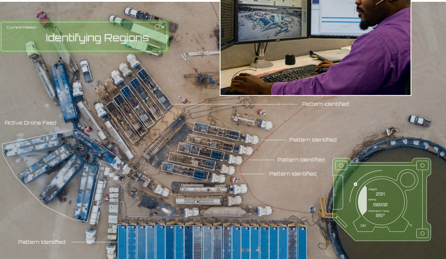
A semiautonomous drone hovering over a hydraulic fracturing fleet scans objects to detect fluid levels on equipment that is difficult to access.
