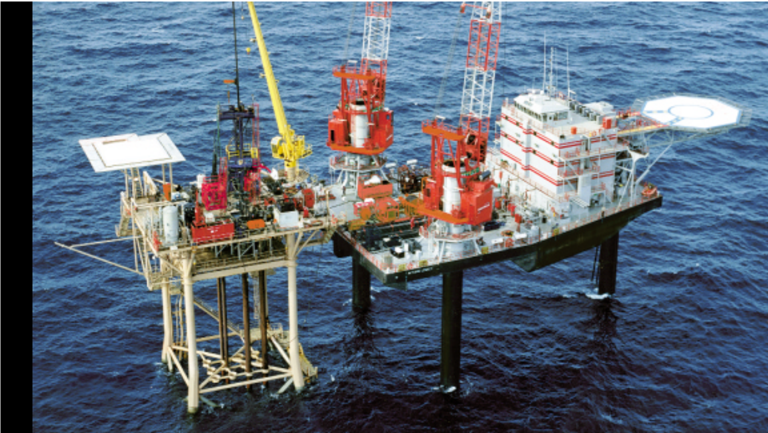
The Dixie Legacy can perform a variety of services, including heavy lifts, construction and pipeline installation support. In addition, the Dixie Legacy can serve as a work platform and staging area for Superior's well intervention services, as it is doing in the above photo.
