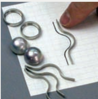
950 palladium wires were annealed and then hand formed.
