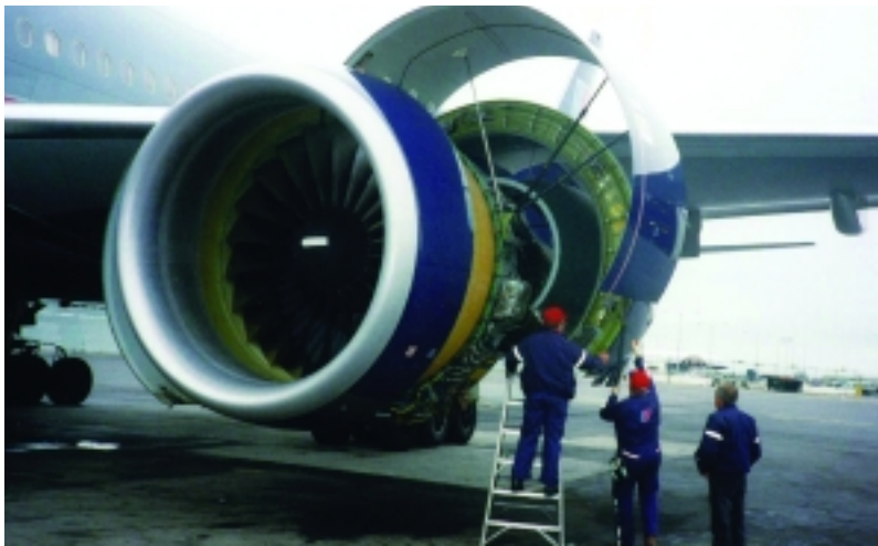
Norco hold-open rods on Boeing 777 Engine Nacelle.
