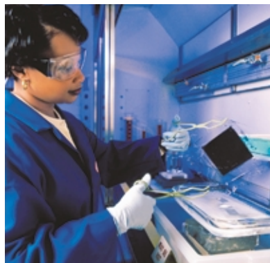
An engineer at DuPont's Fuel Cell Technology Center prepares a catalyst-coated membrane of Nafion® for installation into a fuel cell.
