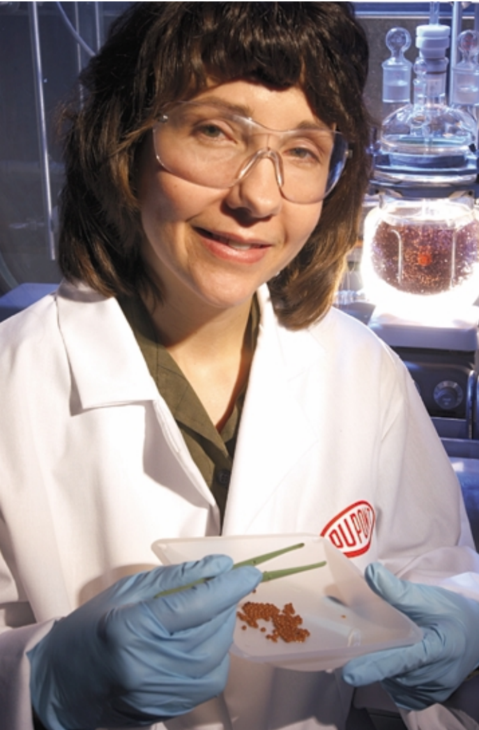
DuPont Chemical Engineer Susan Hennessey uses encapsulated bacteria cells as a biological catalyst to produce DuPont™ Xolvone™, a readily biodegradable solvent for cleaning metals and electronic parts such as computer circuit boards.
