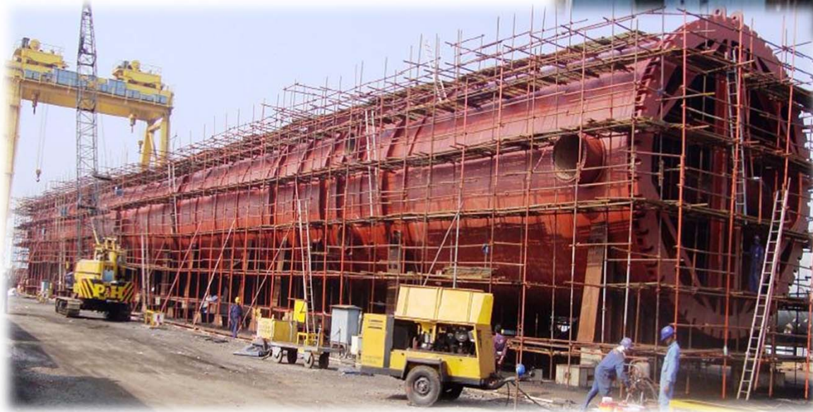
Propylene–Propane Splitter (340' tall – 28' diameter)
