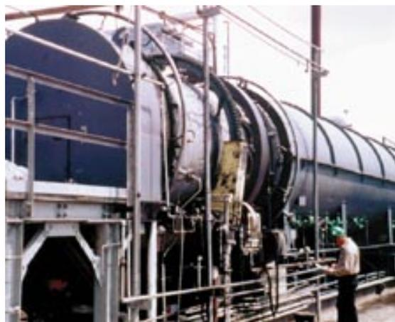
**Technician monitors conditions inside the desorber drum.**
