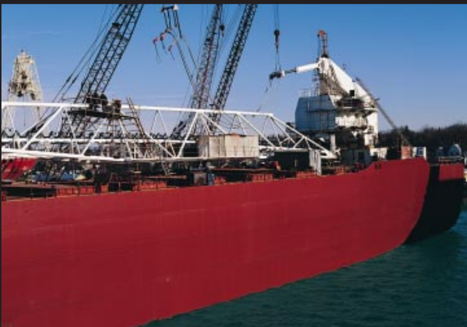
Left: Nearing completion at our Sturgeon Bay shipyard is the Pathfinder , a 604-foot, self-unloading tug/barge that will enter Great Lakes service this spring. Owned by Interlake Steamship Co., Pathfinder was converted into this new configuration from the straight deck bulk carrier J. L. Mauthe .
