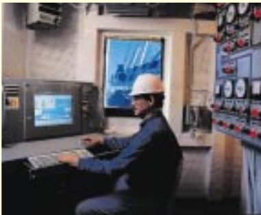
This automated cargo control panel was developed by Manitowoc to upgrade existing Great Lakes vessels.
