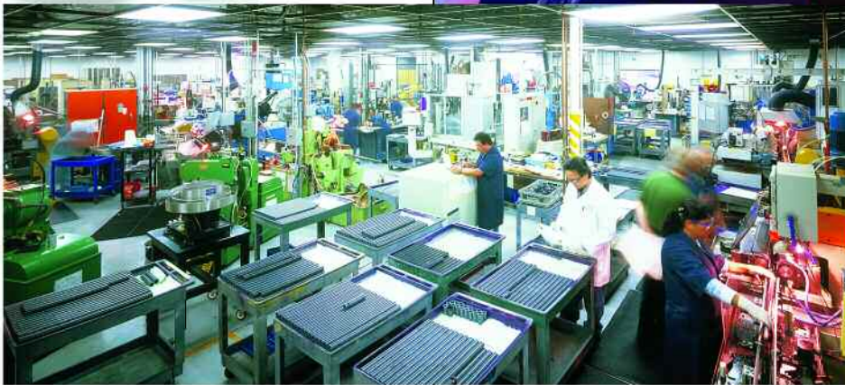
Ceradyne's automated robot-controlled facility in Irvine, California, enables the precision diamond grinding of over 200,000 machined components monthly ( above ).
